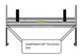
With the super bracket installed on the hanging arms, you can install the nameplate. The nameplate attaches to the top of the hanging arms and super bracket and is held on by 4 black ¼" Torx screws.
